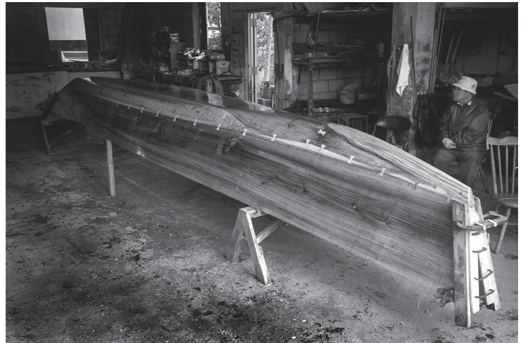
Mr. Ryujin Shimojo looks at the completed hull of the sabani , just prior to turning it over. The wooden dovetail fastening is clearly visible. Photo by Douglas Brooks.
