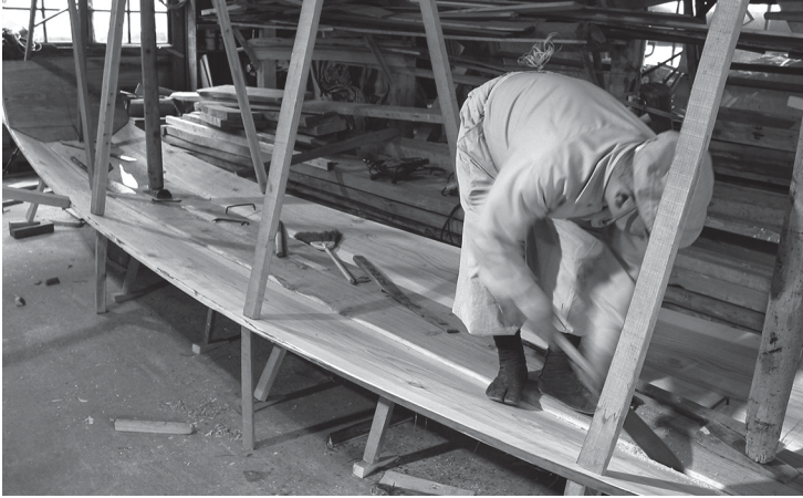
Mr. Seizo Ando of Aomori, Japan building an inshore fishing boat. Ando was the author's fourth teacher, and together they built this boat in the summer of 2003. Ando is fitting the keel and the first plank by running a series of saw cuts through the seam, an essential technique in Japanese boatbuilding. Photo by Douglas Brooks.
