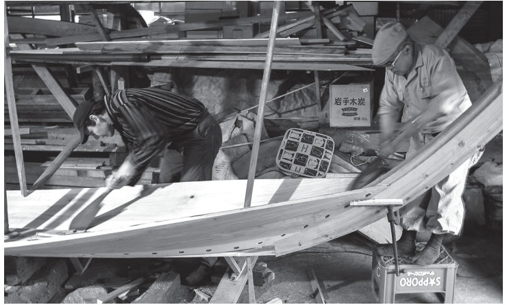
The author and Mr. Ando fitting the seam with handsaws. This technique is called suriawase . Photo by Catherine Wood Brooks.
